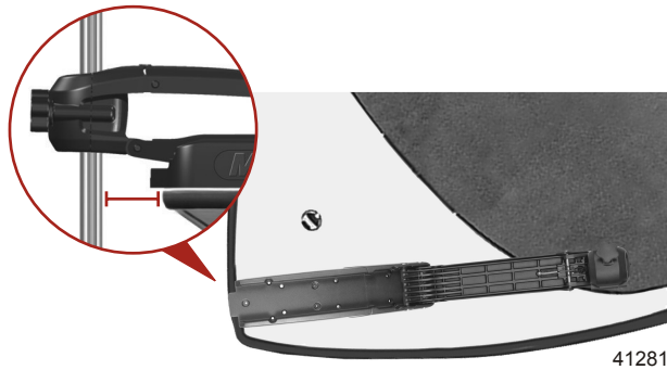
Mount on deck with a 3 in. clearance
