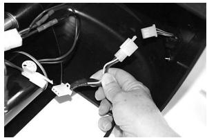
3. Route the wiring harness (the end with one connector) to second switch location. The wiring harness is 24' long. If not long enough, you will need to splice-in more wire. If too long, just coil the extra wire and secure it with cable-ties.
