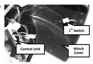
2. One end of the wiring harness has two connectors. Connect them to the switch on winch housing and to the control unit.
