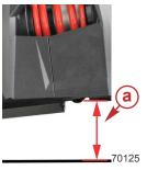
a - Distance between the boat deck and the outside surface of the mounting bracket.
