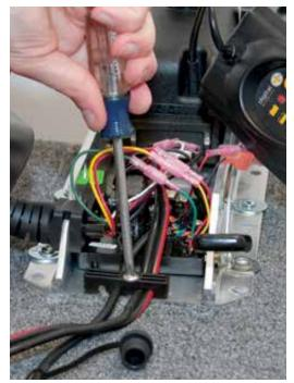
16. Loosen the cable strain relief that is secured to the base of the motor and install the i-Pilot Link controller steering cable into the open strain relief slot. (Figure 29)
