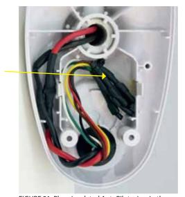
FIGURE 21 Place insulated AutoPilot wires in the bottom center of the control box as shown.
