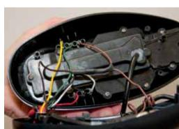
FIGURE 18 Insert AutoPilot wires into terminal holder
