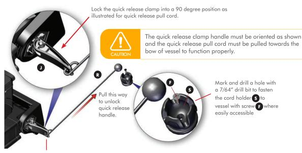
Fasten the end of R quick release pull cord to quick release clamp handle by tying them together using a knot.
