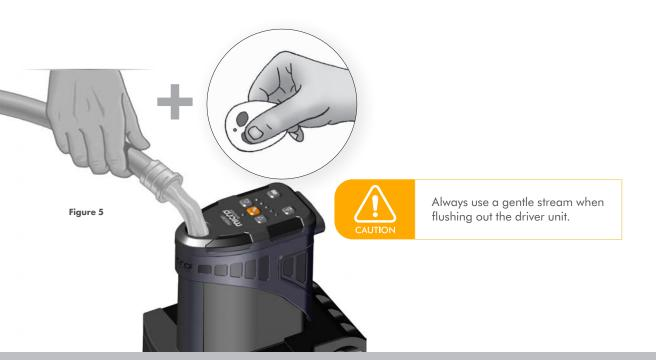
With the spike removed, double tap the Key Fob or Dash Switch DOWN button to run the unit a full 30 seconds while simultaneously flushing with low flow water. Repeat as needed to clean all debris from spike pocket mechanical parts.
